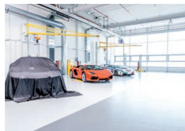
Large windows made of triple-layer polycarbonate mounted with double chambers and filters to reduce refracted sunlight ensure proper solar illumination and a high level of thermal insulation.
